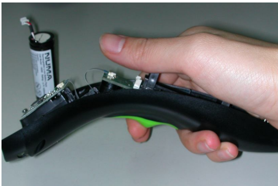
7. Hold the trigger for 1min to releaseremaining power
