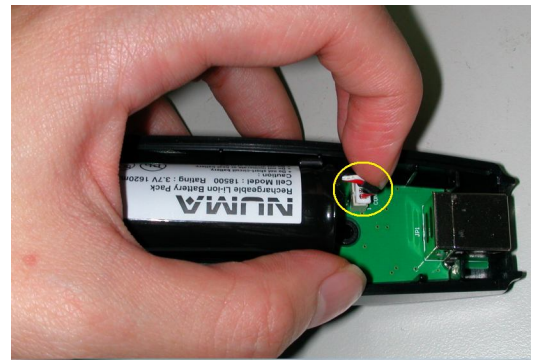
6. Disconnect the battery from PCB board
