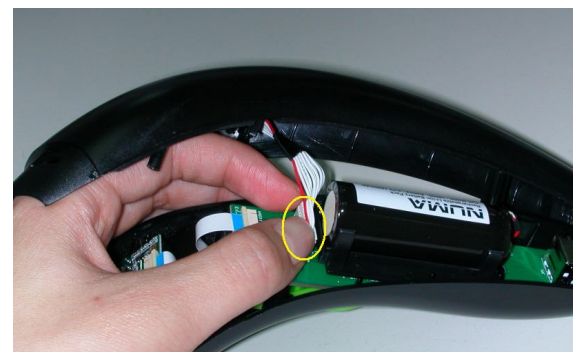
6. Disconnect the battery from PCB board
